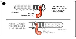
Unscrew the hex on the remote lever using a 4mm hex key, and lightly grease the clamp I.D. (see fig. 4).
